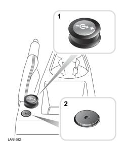
The auxiliary connector is situated at the rear of the centre console.
